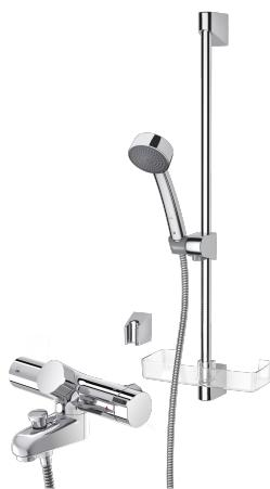
Bath and shower faucet that reacts quickly and precisely to the changes of water pressure and keeps the water temperature as selected. Suited to places where there are several water outlets and the network always contains plenty of hot water. The temperature adjustment knob is equipped with a temperature limiter which can be bypassed by pushing a button.
